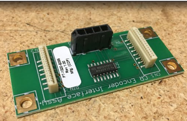
PT-1320-E065 | CR Encoder Interface Board
